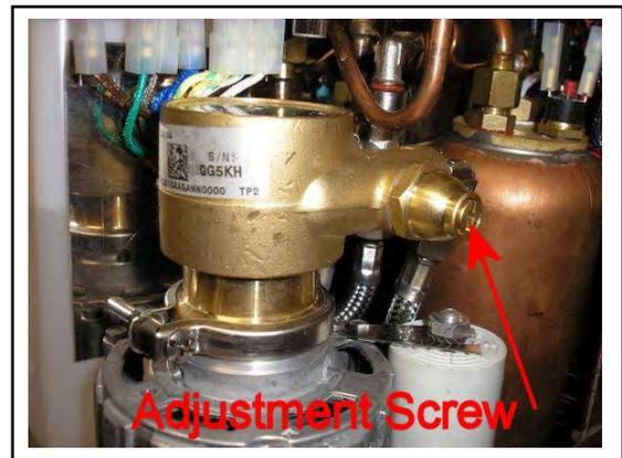
The recommended setting is 9 bar. The pressure may vary based on your line pressure or if you are using the machine in plumbed mode versus reservoir mode. When plumbed in it is normal to see some pressure shown in the pump gauge when it is not being used which is showing the line pressure to the machine.
