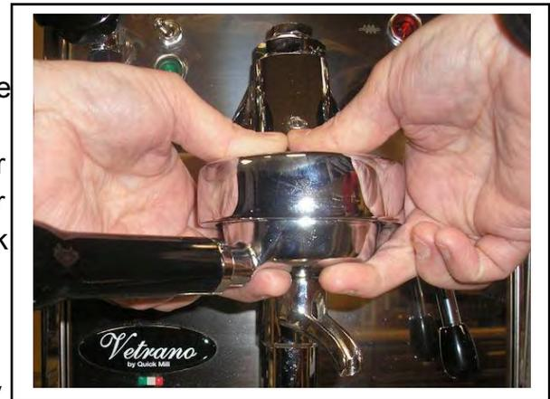
Maintenance Tip: Replacing the gasket on a yearly basis will make the replacement procedure much easier. There are also benefits to having a new gasket. It will provide a better seal for a better espresso extraction and it also enables you to be able to remove the shower screen without ruining the gasket to provide for better cleaning which will result in better tasting shots.
