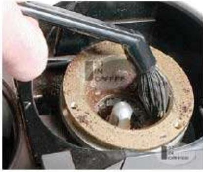
Without turning the burr, use a stiff brush (the brewhead brush works great for this task) and clean that area out. A plastic or wooden tool will also be useful in some cases. After the debris is removed from the burr, either turn Rocky upside down and shake it or use compressed air to blow out the grinding area—do so outside and use eye protection as coffee will go everywhere!
