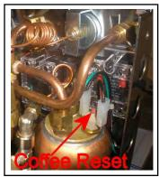
With the machine unplugged, firmly press the red reset button shown in the attached pictures.
